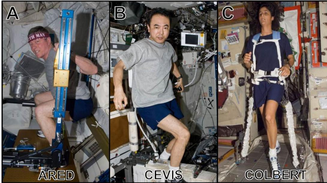
**Figure 4.** Images of astronauts exercising on equipment currently used aboard the ISS. **A:** Advanced Resistance Exercise Device (ARED), **B:** Cycle Ergometer with Vibration Isolation and Stabilization System (CEVIS), and **C:** Combined Operational Load Bearing External Resistance Treadmill (COLBERT). Images retrieved from <http://www.nasa.gov/>.
